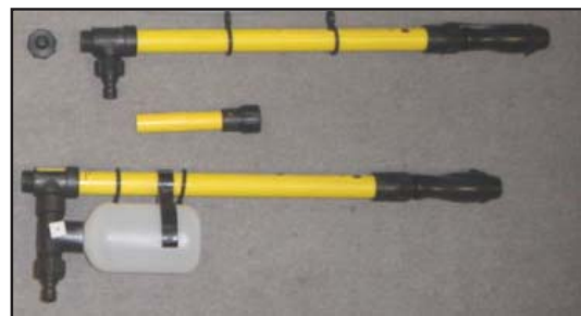
Top pump: Standard (water only) Bottom pump: Foam capability
